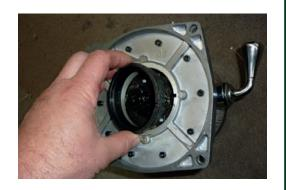
4. Undo and remove 10 Allen head bolts that hold the gearbox housing to the drum support housing and rotate the drum support housing to the desired location.
