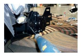
17. Fit winch mounting cradle between chassis brackets using M12 hardware, align rear protection plate mounting points with front holes of factory protection plate and tighten all bolts.
