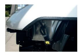
9. Trim guard liners along line as shown and remove square section adjacent to edge of bumper as shown.
