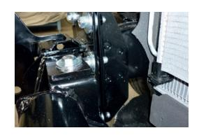
16. Using holes in strengthening brackets as a guide drill two horizontal holes through chassis and secure using M10 x 100mm bolts, flat washers, crush tubes, spring washers and nuts.
