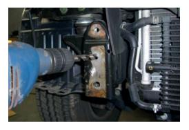
13. Insert nut plate into front of chassis and attach mounting bracket using M12 bolts, spring washers and flat washers provided.
