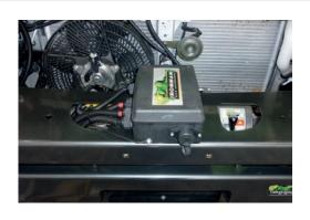
12. Connect three colour coded cables to the corresponding poles on winch motor.
