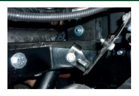
13. Refit plastic bumper reinforcement and top section of bumper bar.
