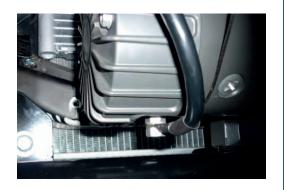
14. Run the positive and negative battery cables into the engine bay taking care to secure cables away from any sharp or moving objects.
