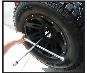
Step 2. Remove the (2) top right hand 13mm hex bolts from the spare tire mount.
