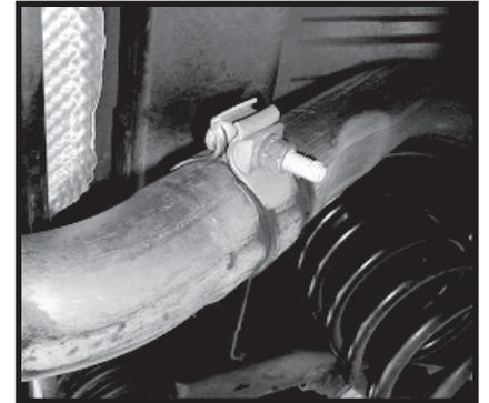
Step 2. Remove the muffler from the (2) rubber isolator mounts. A spray lubricant may be needed.
