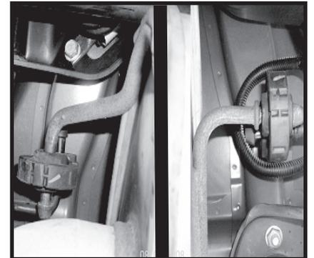
Step 3. Install the new exhaust by first attaching the muffler to the rubber isolator hangers.
