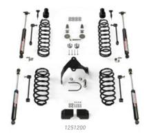
The TeraFlex JK/JKU: 3" Coil Spring Base Kit includes just the basic lift components only and doesn't have the driveability of a full suspension system. Requires longer preset or adjustable control arms and adjustable front track bar to correct suspension geometry.
