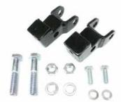
Move the canister away from the spring pad with the TeraFlex TJ/LJ: Rear Lower Shock Extension Kit. Simply installs into the factory shock location. This kit eliminates shock body damage during extreme suspension articulation as well as allows for custom pinion angle adjustment and axle rotation on lifted TJ/LJ Wrangler models.
