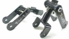
TeraFlex Revolver Shackles feature a unique design that hinges and rotates to allow the leaf springs to flex and compress without additional spring stress. These self-supporting shackles fold against themselves on level ground.
