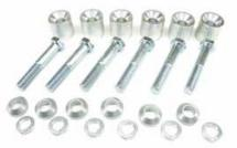
These TeraFlex TJ/LJ: Transfer Case Lowering Spacer Kit lowers the transfer case to reduce driveshaft vibration caused by a ride height 2" or more above stock - especially on TJ/LJ Wrangler models without either a slip yoke eliminator kit or adjustable control arms.
