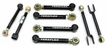
The TeraFlex TJ/LJ: 8-Arm Alpine Flexarm Kit provides complete alignment adjustability for maximum performance on TJ/LJ Wrangler models with 0-4" lifts. Uses factory control arm brackets. Can be added to any existing suspension lift.
