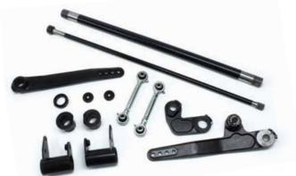
This system incorporates two torsion bars: the "Street" bar is tuned for a stable ride and heavy-duty highway handling, while the "Trail" bar is tuned to control body sway and lean during side hill and off-camber situations with full off-road articulation.
