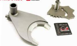
The TeraFlex TJ/LJ: NP231-J 2Low 2WD Low-Range Shift Sector Kit adds a lowrange 2WD/RWD (two-wheel-drive/rear-wheel-drive) option to the TJ/LJ Wrangler models' NP231-J transfer case's standard low-range shift pattern.
