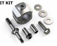
The TeraFlex JK/JKU: Steering Stabilizer Relocation Mounting Bracket Kit moves the steering stabilizer up nearly 2.5" to help reduce damage to the stabilizer shaft or body. The 6061-T6 aluminum clamp and forged 10.9 grade stud reposition the stabilizer to reduce "tie rod roll" that causes a dead spot of un-resisted movement in the steering.
