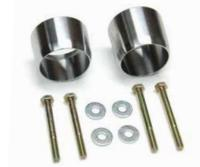
The TeraFlex 2012-2018 JK/JKU: Exhaust Spacer Kit is required for all 2012-2018 JK/JKU Wrangler models with 2.5" or more lift. Prevents contact between the front driveshaft and the exhaust crossover pipe during suspension down travel. Installs between the exhaust header flanges and the crossover pipe flanges to move the crossover pipe rearward for proper driveshaft clearance.
