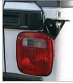
Simply install the TJ/LJ  $\mid$  YJ  $\mid$  CJ: CB Antenna Mount Kit between the brake light and the body. Available for driver or passenger side. Drilling is optional, but not required.
