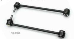
The TeraFlex JK/JKU: Rear Sway Bar Link Kit reduces clearance issues between the tire and rear sway bar. The sealed narrow shoulder tie rod type ball socket on the upper link maximizes tire clearance, while the sealed ball socket on the lower link provides precise and immediate reaction during sway bar loading thus eliminating excess play. Sold in pairs.
