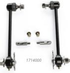
The upper sway bar link end has an OEM quality polyurethane shoulder ball and socket for silent operation, long-term durability, and zero maintenance. The lower sway bar link end features a large polyurethane ball that slides over a stainlesssteel pin for easy sway bar link removal.
