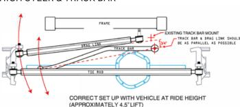
Properly aligned axle components will help eliminate bump steer and other steering issues common on lifted vehicles with a high steer system. The key is to make the track bar and drag link as parallel as possible.
