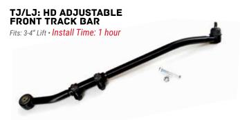
The TeraFlex TJ/LJ | ZJ | XJ: HD Adjustable Front Track withstands abusive side loads experienced when steering off-road to drastically improve steering response and handling. Allows lateral adjustment of the axle for proper axle alignment as well as full suspension travel. Recommended for 3-4" lifts.
