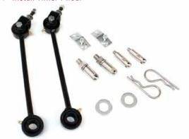
TeraFlex TJ/LJ: Front Sway Bar Quick Disconnects are the industry leader thanks to their ease of use. The Sway Bar Links quickly disconnect and swing up out of the way for unrestricted axle articulation during off-roading. While connected for street use, the link provides immediate reaction during sway bar loading to eliminate excess play. This results in improved lateral control and steering response compared to the stock rubber sway bar link bushings.
