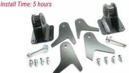
TeraFlex TJ/LJ: HD Hemi V8 Motor Mounts are laser cut from 1/4" steel to withstand the Hemi V-8's horsepower and torque, while the Clevite rubber bushings provide superior vibrations control as well as strength and dependability to prevent shearing from the frame under load.
