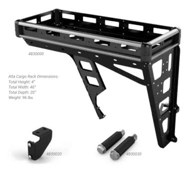
The TeraFlex JKU 4-Door: Wasatch Rear Cargo Rack provides additional storage options to organize and secure cargo. Inspired by the Nebo Roof Rack System, the rear cargo rack provides universal accessory mounting compatibility. The extruded aluminum rails utilize the industry standard 10-series T-slot mounts that readily accept available mounting hardware for small accessories or recovery equipment.
