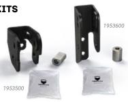
These TeraFlex JL/JLU: Front Track Bar Axle Bracket Kits correct steering geometry, eliminate bump steer, and other front-end issues on lifted Jeeps. The TeraFlex JL/JLU: Rear Track Bar Axle Bracket Kit corrects vehicle roll center, restores factory handling, and reduces body roll in lifted Jeeps.
