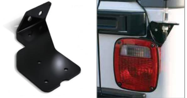
Simply install the TJ/LJ | YJ | CJ: CB Antenna Mount Kit between the brake light and the body. Available for driver or passenger side. Drilling is optional, but not required.
