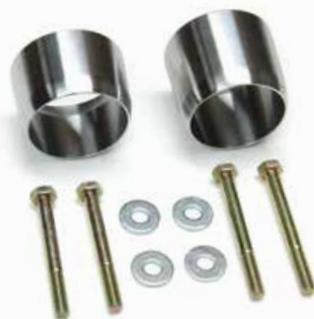
The TeraFlex 2012-2018 JK/JKU: Exhaust Spacer Kit is required for all 2012-2018 JK/JKU Wrangler models with 2.5" or more lift. Prevents contact between the front driveshaft and the exhaust crossover pipe during suspension down travel. Installs between the exhaust header flanges and the crossover pipe flanges to move the crossover pipe rearward for proper driveshaft clearance.
