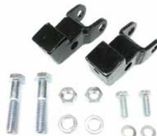
Move the canister away from the spring pad with the TeraFlex TJ/LJ: Rear Lower Shock Extension Kit. Simply installs into the factory shock location. This kit eliminates shock body damage during extreme suspension articulation as well as allows for custom pinion angle adjustment and axle rotation on lifted TJ/LJ Wrangler models.
