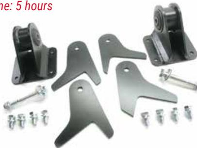
TeraFlex TJ/LJ: HD Hemi V8 Motor Mounts are laser cut from 1/4" steel to withstand the Hemi V-8's horsepower and torque, while the Clevite rubber bushings provide superior vibrations control as well as strength and dependability to prevent shearing from the frame under load.
