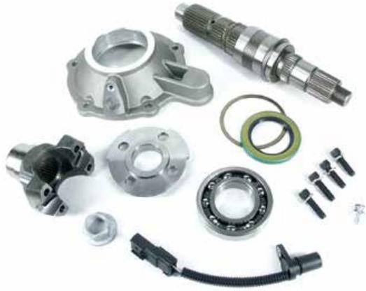
The TeraFlex TJ/LJ: NP231 Extreme Short Shaft Kit is what short-wheelbase TJ/LJ Wrangler owners have been dreaming about for decades. Not only does the Extreme Short Shaft Kit improve on strength, but it also increases driveshaft length by up to 7" over a stock application. This kit is also more than 3" shorter than a standard Slip Yoke Eliminator Kit and 1.5" shorter than an ATLAS II. Speedometer readings are transferred through a tone ring and electronic sensor.
