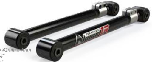
Tube Diameter & Wall = 42mm x 4mm
