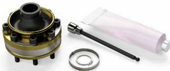
The TeraFlex JK/JKU: Rzeppa High-Angle Factory Replacement CV Joint Kit replaces a worn or damaged factory Rzeppa CV joint and driveshaft without resorting to an expensive aftermarket U-joint upgrade. Allows angles up to 15 degrees. The high-angle CV housing reduces boot failure associated with 3" or more lift.
