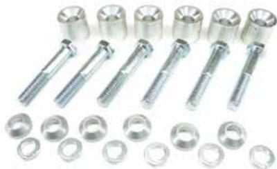
These TeraFlex TJ/LJ: Transfer Case Lowering Spacer Kit lowers the transfer case to reduce driveshaft vibration caused by a ride height 2" or more above stock – especially on TJ/LJ Wrangler models without either a slip yoke eliminator kit or adjustable control arms.
