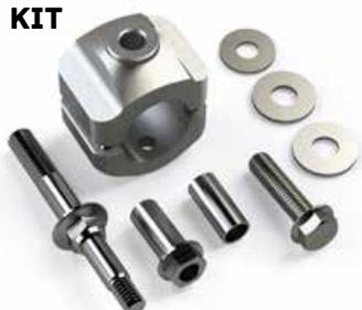
The TeraFlex JK/JKU: Steering Stabilizer Relocation Mounting Bracket Kit moves the steering stabilizer up nearly 2.5" to help reduce damage to the stabilizer shaft or body. The 6061-T6 aluminum clamp and forged 10.9 grade stud reposition the stabilizer to reduce "tie rod roll" that causes a dead spot of un-resisted movement in the steering.
