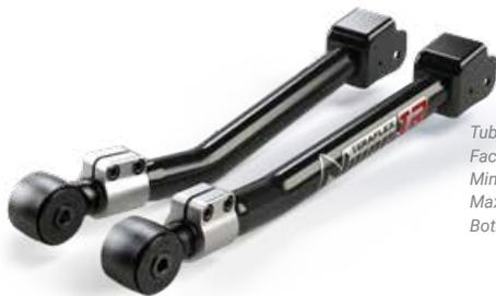
Tube Diameter & Wall = 42mm x 4mm
