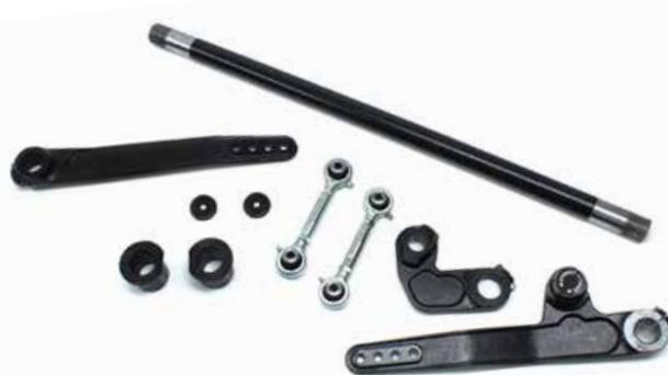
A simplified version of our Dual-Rate ST Front Sway Bar System, the Single-Rate ST Front Sway Bar System features only the heavy-duty "Street" torsion bar (with Easy Engagement Knob) for superior highway handling.
