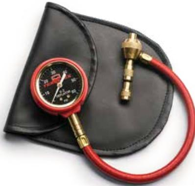
Quickly and accurately lower your tire air pressure for trail comfort and performance with the TeraFlex EZ-Deflator Kit. The simple 2" dial gauge gives accurate pressure reading while airing down to take the guesswork out of the process. The sealed bourdon tube construction is calibrated before final assembly and is unaffected by changes in altitude, humidity, or temperature. Mechanical accuracy rating certified to ±2%.
