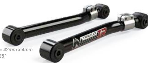
Tube Diameter & Wall = 42mm x 4mm
