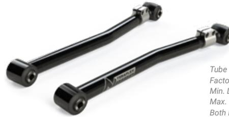
Tube Diameter & Wall = 42mm x 4mm
