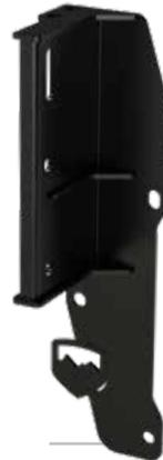
The heavy-duty JK/JKU: Alpha Hi-Lift Jack Mount provides a safe, quiet, and secure mounting point for a Hi-Lift Jack. The 3/16" thick laser cut and powder coated bracket bolts to the Alpha HD Hinged Spare Tire Carrier for unshakable stability. This mount also incorporates a built-in CB antenna mount as well as an off-road flag mount for those sand dune trips.
