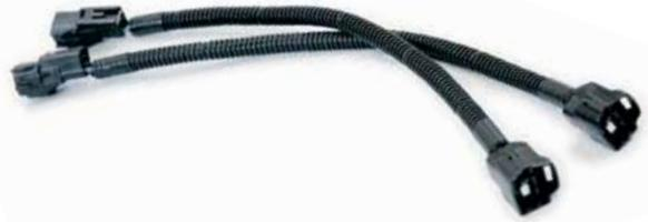
Retain your factory fog lights with "short" style bumpers with this TeraFlex TJ/LJ: Fog Light Extension Wire Kit. The simple extension wire uses factory style connectors for a clean installation.
