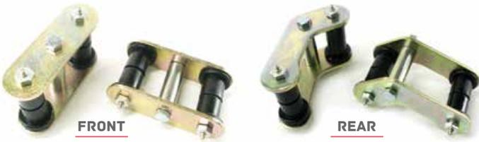
Replace your flimsy stock shackles with these TeraFlex YJ: HD Shackle Kits. Our HD Front Shackles and HD Rear Kickback Shackles are constructed from 1/4" steel with an attractive zinc plating to resist corrosion. The bolted cross brace increases rigidity and strength and won't bend and become a safety hazard.
