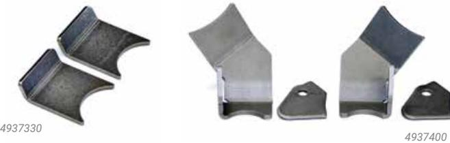
These weld-on TeraFlex JK/JKU: Lower Flexarm Skid Plate Kits strengthen the lower control arm assembly against bending, while protecting the arms from damage. The CNC cut brackets are constructed from 1/4" thick steel. Available for front lower and rear lower control arms. Sold in pairs with all necessary hardware.
