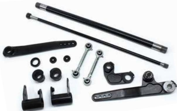
This system incorporates two torsion bars: the "Street" bar is tuned for a stable ride and heavy-duty highway handling, while the "Trail" bar is tuned to control body sway and lean during side hill and off-camber situations with full off-road articulation.
