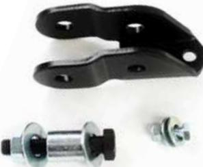
The Spacer Lift Rear Track Bar Frame Bracket Kit restores the track bar to its natural position without binding or interference with other components on JK/JKU Wrangler models with a 2.5" Performance Spacer Lift Kit.
