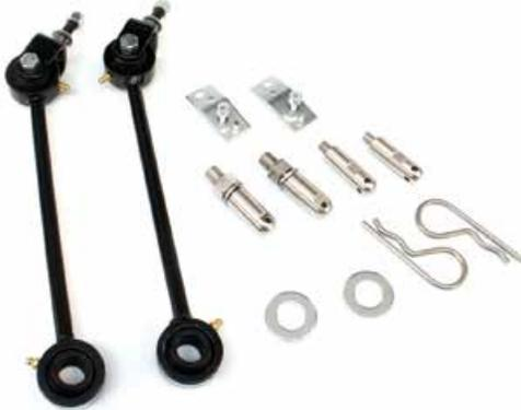
TeraFlex TJ/LJ: Front Sway Bar Quick Disconnects are the industry leader thanks to their ease of use. The Sway Bar Links quickly disconnect and swing up out of the way for unrestricted axle articulation during off-roading. While connected for street use, the link provides immediate reaction during sway bar loading to eliminate excess play. This results in improved lateral control and steering response compared to the stock rubber sway bar link bushings.
