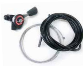
The TeraFlex TJ/LJ | YJ | CJ: Hand Throttle Cable Kit provides constant idle or speed when off-roading, which is especially useful when the gas, clutch, and brake are needed together. Works with all carburetor and fuel injection engines with a cable-operated throttle. Does not fit engines with drive-by-wire throttle systems. Intended for off-road use only and NOT as a "cruise control" device.
