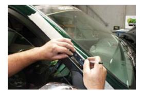
11. Apply silicone sealant to holes. Insert mounting plugs and attach mounting bracket to pillar using self tapping screws provided.
