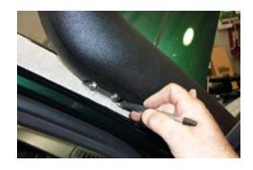
10. Hold snorkel bracket in position and mark four mounting holes on pillar. Drill mounting holes to 7.5mm.
