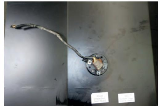
18. Refit filter to fuel pick up and install assembly to fuel tank making sure the pick up is close to but not touching the bottom of the fuel tank.
