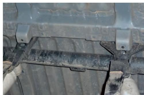
11. Bend bracket on cross member up and forwards as shown to allow clearance for new tank.
