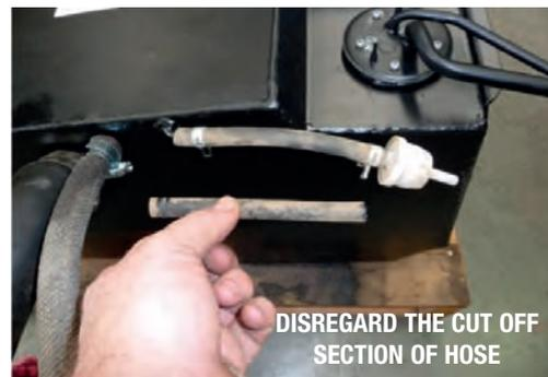
20. Lift fuel tank into position in vehicle and secure front mount to round cross member between upper shock absorber mounts.
