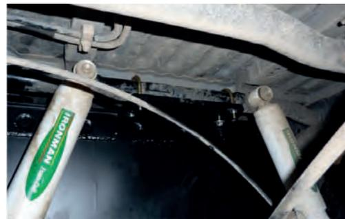
21. Raise and support rear of fuel tank so that mounting points are pushed against corner gussets of chassis. Centralise fuel tank and drill holes through chassis on each side using mounting holes in fuel tank as a guide.
