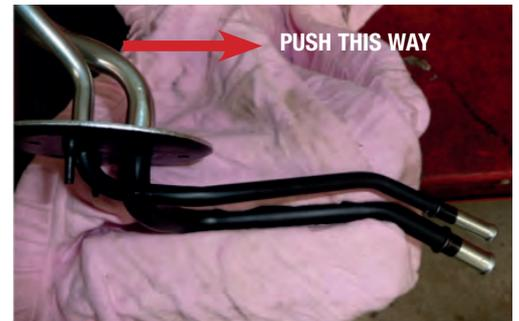
17. Install fuel sending into new tank making sure the float clears the bottom of the tank.
