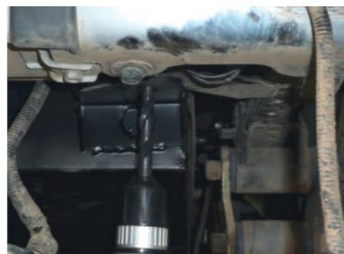
22. Rust proof holes drilled in previous step and secure rear mounts to chassis using bolts, washers and nuts supplied.
