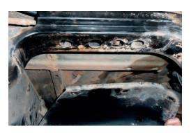
3. Bracket on chassis for rear tank strap will need to be modified so that opening is 36mm wide. This will allow new tank strap to be installed.
