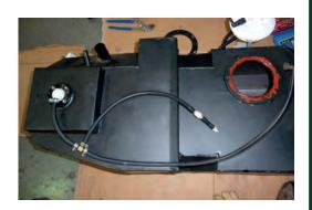
6. Remove heat shield from front of original fuel tank and fit to new tank.
