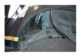
3. Disconnect fuel filler hose, fast fill breather and tank breather hoses.
