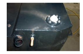
9. Refit tank to vehicle. As tank is being lifted in position reconnect fuel sender wiring and reattach fuel hoses to fuel pipes.
