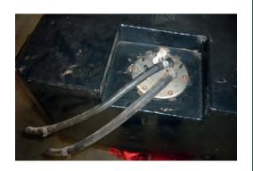
8. Fit rollover valve and barb fitting supplied to new tank as shown.
