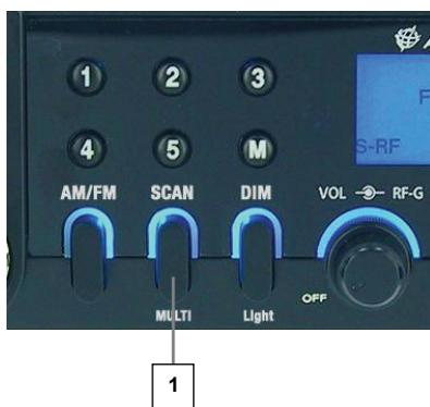
Before You can use Your new CB radio the first time, You should program it to the correct country code. Press the SCAN/Multi-Mode button (1) while the device is still off and switch on your radio while keeping the button pressed. Release the button. Now the multi standard choice 01 to 05 will appear in the display. Select the mode for Your country by turning the channel switch (see the following table and our radio passport). Switch the radio off and on again after selection of the country code.
