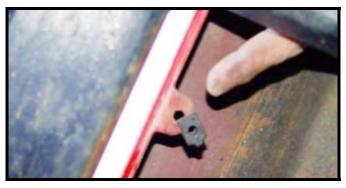
**Step 5:** Position armor onto lower side rocker panels. Make sure that it is evenly spaced before applying any pressure to armor. When satisfied with placement apply pressure to all areas to properly secure armor to vehicle. Secure bottom of rocker guards with hardware supplied.
