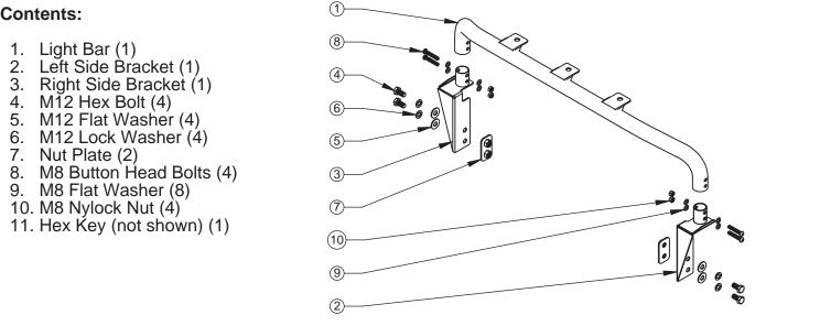
07-09 JK: Locate the two frame mounting holes behind the bumper on the left side of the vehicle. Slide 1. the Nut Plate behind the two holes. Use the M12 Hex Bolts, Lock Washers and M12 Flat Washers to secure the Left Side Bracket to the frame as shown. Do not fully tighten the bolts at this time. Repeat for right side.
