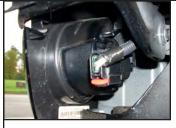
**Step 8.** Reinstall the bulb/socket assembly, remembering to rotate it to secure it to the housing.
