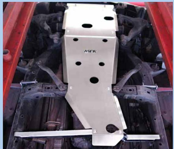
Transmission (Gear) skid plate - Land Cruiser 125 SWB
